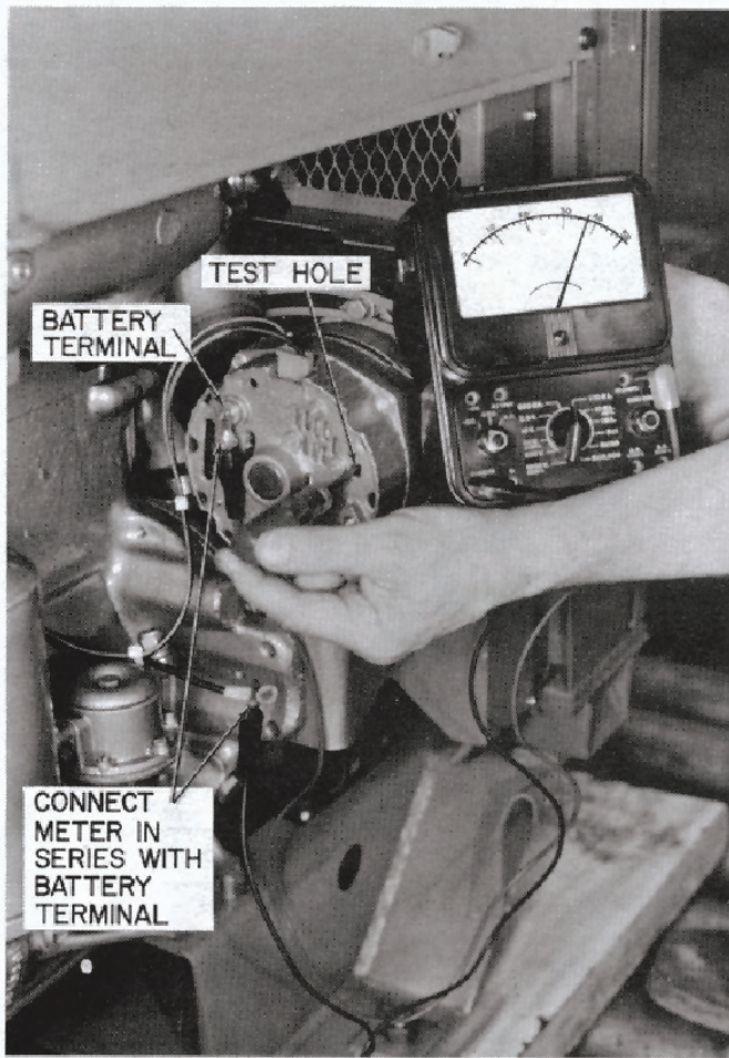
TESTING ALTERNATOR OUTPUT
