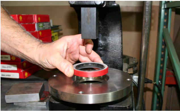
Figure 7.6 Press in oil seals
