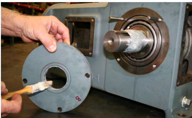
Figure 7.16 Lubricate sleeve and oil seal
