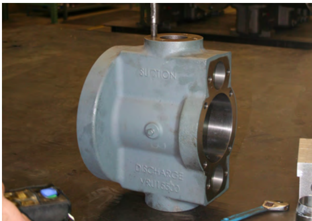
Figure 7.37 Inspect an clean cylinder
