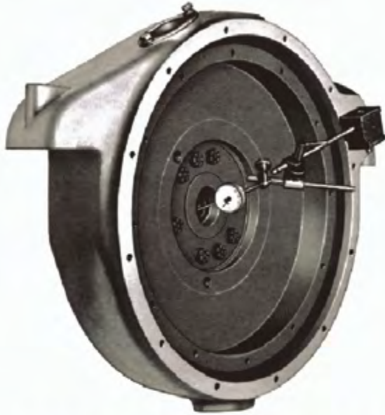
CHECKING PILOT BEARING BORE RUNOUT
