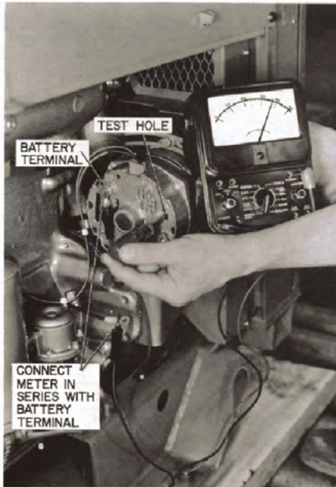
TESTING ALTERNATOR OUTPUT
