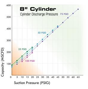
Charts based on natural gas with a specific gravity of 0.65
