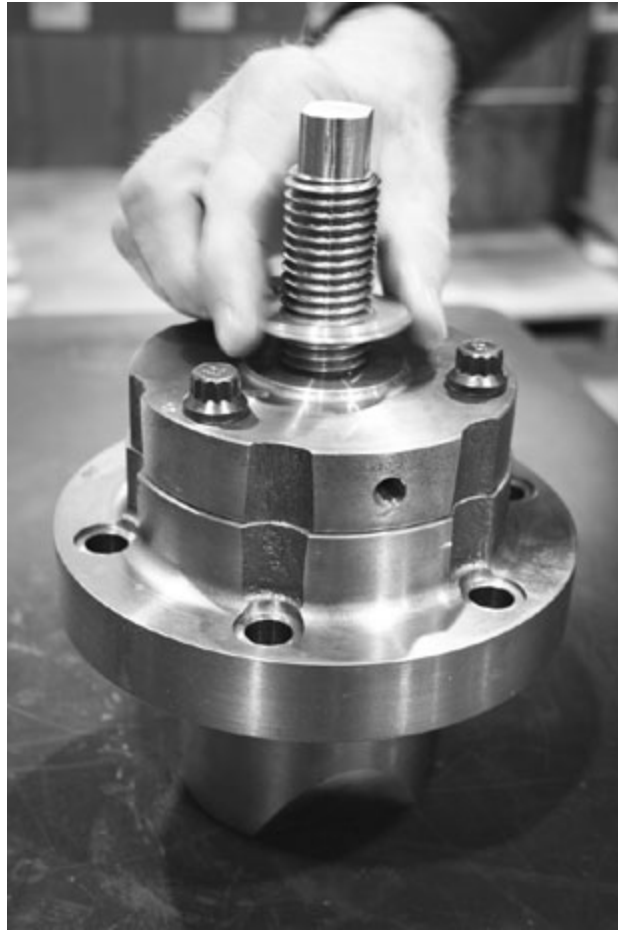
12. Insert the first of two (2) VVCP adjusting stem cover gaskets (VRC27105).
