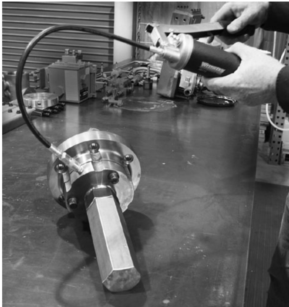
19. Using a grease gun, fill the VVCP with grease via the grease zerk.
