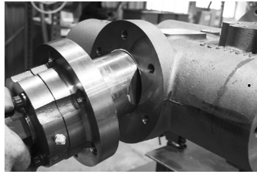
2. Insert VVCP into cylinder making sure the flats on the VVCP head align with the valve ports.
