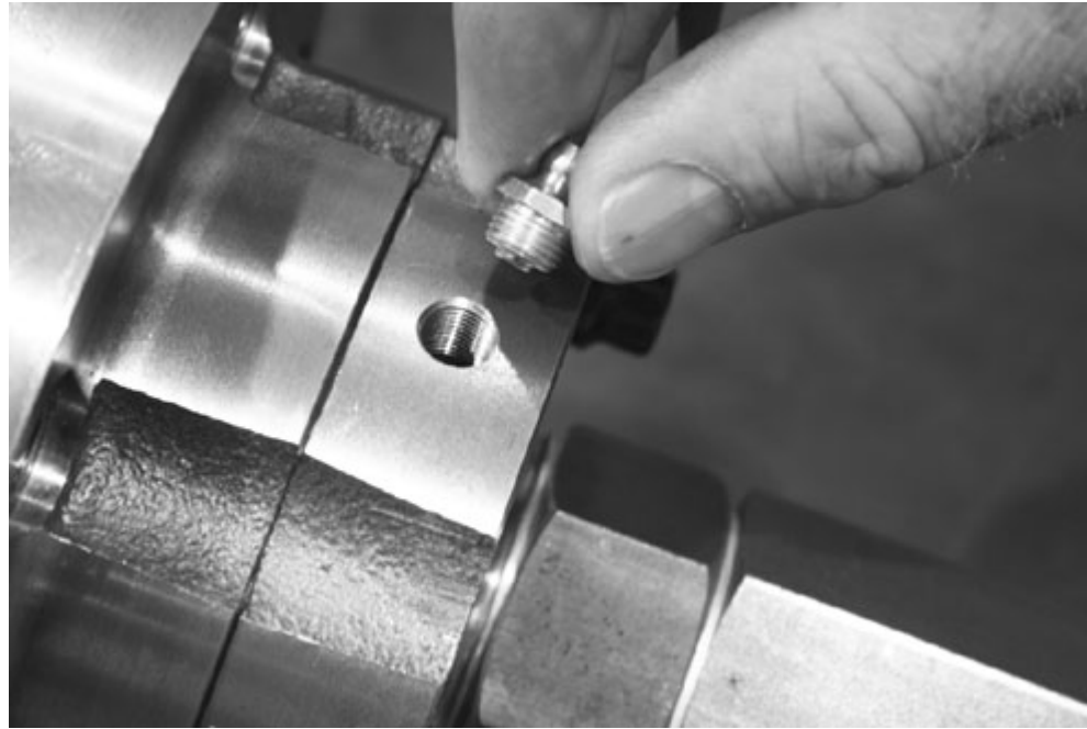
18. Insert VVCP grease zerk (VRC27109) into the hole located in the VVCP pocket cover.
