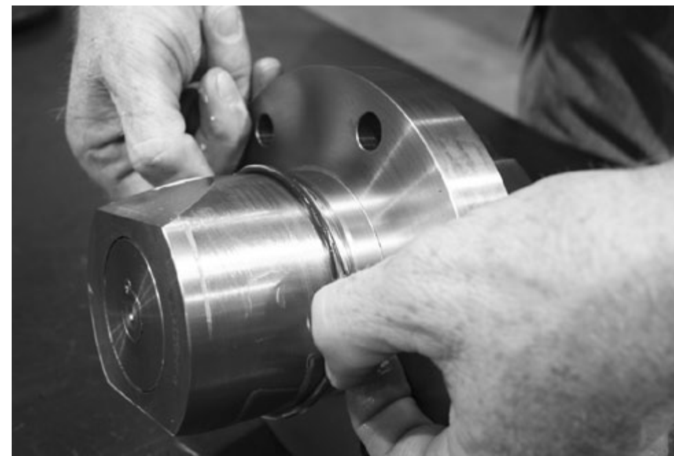
16. Lubricate the crank-end outer head O-ring (VRC27101).
