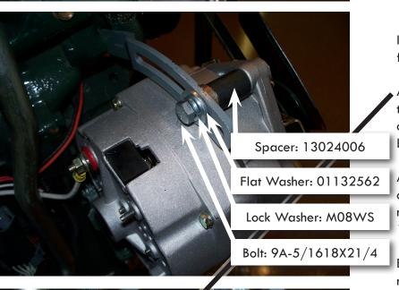
Install new spacer and hardware from kit and install to alternator.
