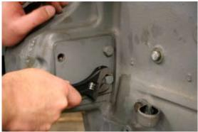
5. Remove block off plate from crankcase front cover and replace with block off plate containing 1/4"NPT hole
