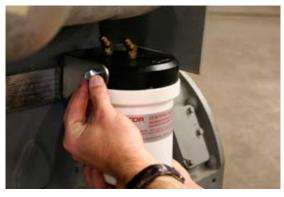
4. Reattach filter to mounting bracket. (Use Loctite 271 or equivalent, not included, for head fitting threads.)
