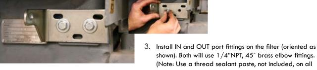
shown). Both will use 1/4"NPT, 45° brass elbow fittings. (Note: Use a thread sealant paste, not included, on all pipe threads and fittings. Use care not to get sealant into passages of hoses or fittings. Do not use Teflon tape.)
