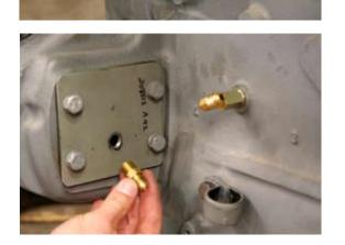
7. Attach straight brass fitting with 1/4"NPT-to-5/16" tube fitting to 1/4"NPT hole in block off plate.
