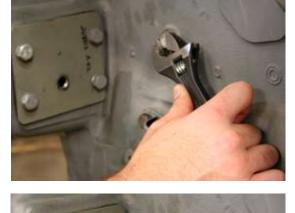
6. Remove plug from pressurized port located on left side of engine block. Replace plug with M10x1-to-1/8"NPT adapter. Attach 90° brass elbow with 1/8"NPT-to-5/16" tube fitting to adapter.
