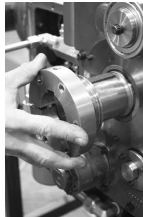
5. Slip the sheave onto the shaft with the belt grooved side towards the frame.
