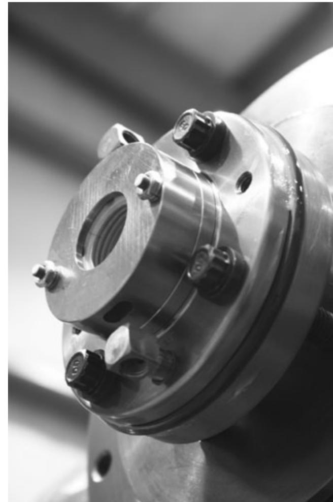
17. Use the same procedure for the fitting for the "vent" hole. The "vent" hole of the fitting will be facing DOWN. The cylinder is now ready to be attached to the frame.
