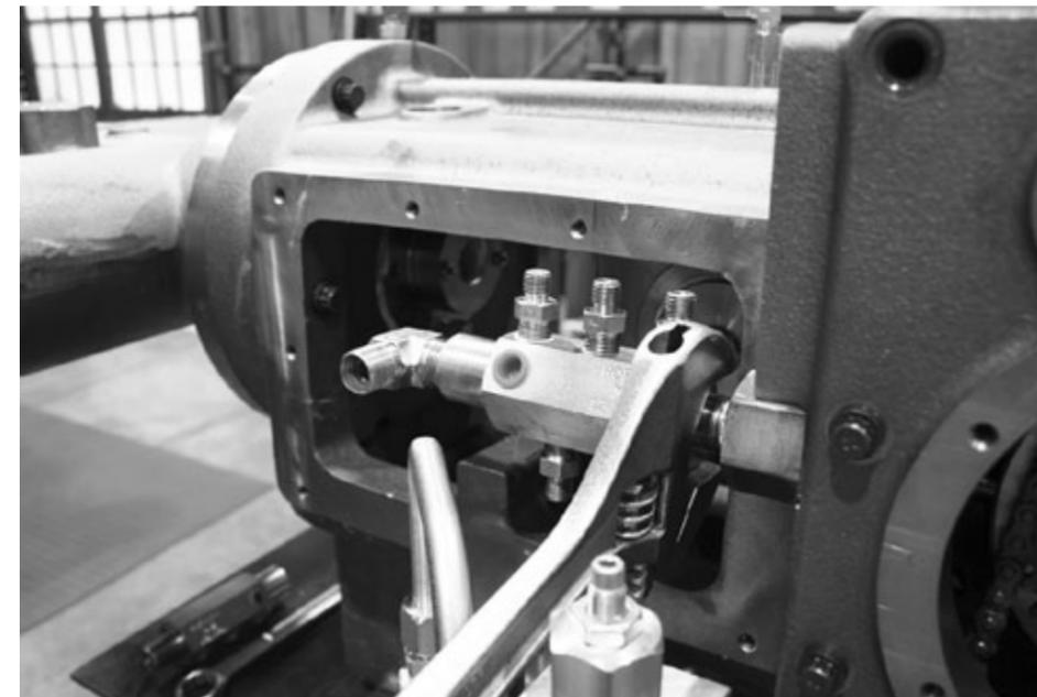
3. Install fitting (VRC28853) in the outlet of the filter bracket with 90° outlet printing out from the accessory end.
