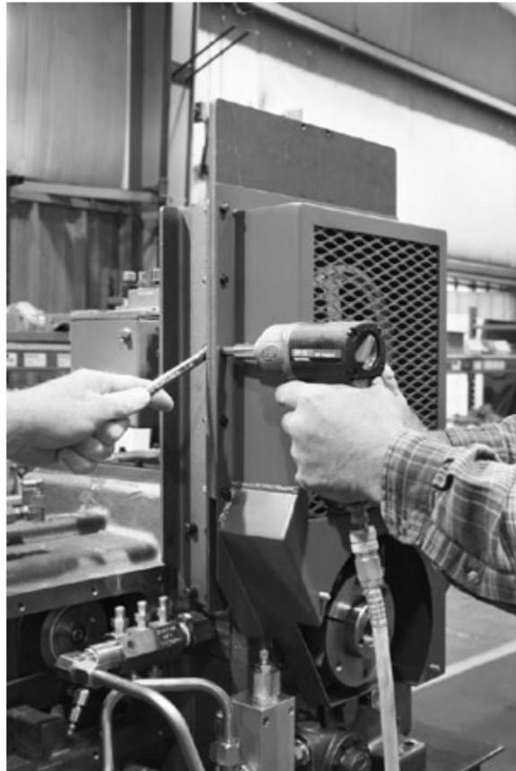
2. Mount the belt guard (VRC28480) onto the mounting plate, replace and tighten screws.
