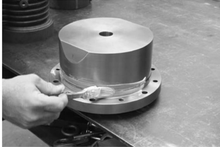
1. Clean crank-end head making sure the crank-end O-ring groove is free of any debris.
