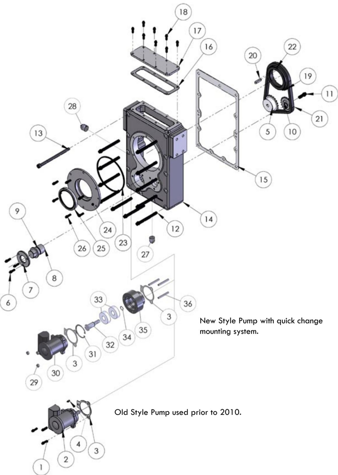
New Style Pump with quick change mounting system.
