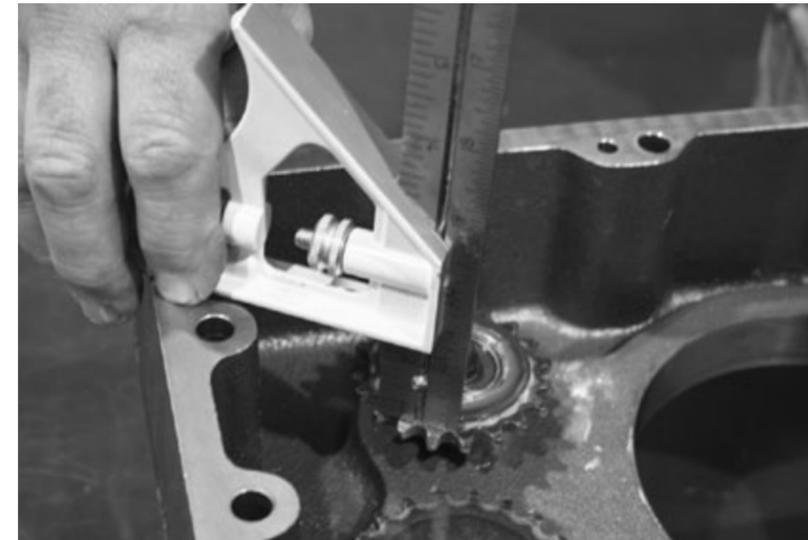
5. From the inside of the housing, install the key to the frame oil pump shaft (VRC28236). Then slide the oil pump drive sprocket (VRC28232) onto the shaft. DO NOT TIGHTEN. You must do a sprocket alignment first before you tighten.
