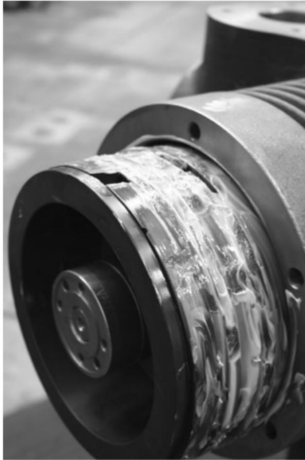
4. Stagger the piston ring gaps and then compress the piston rings with your fingers as you slide the piston rod assembly into the cylinder. Be careful not to pinch your fingers.
