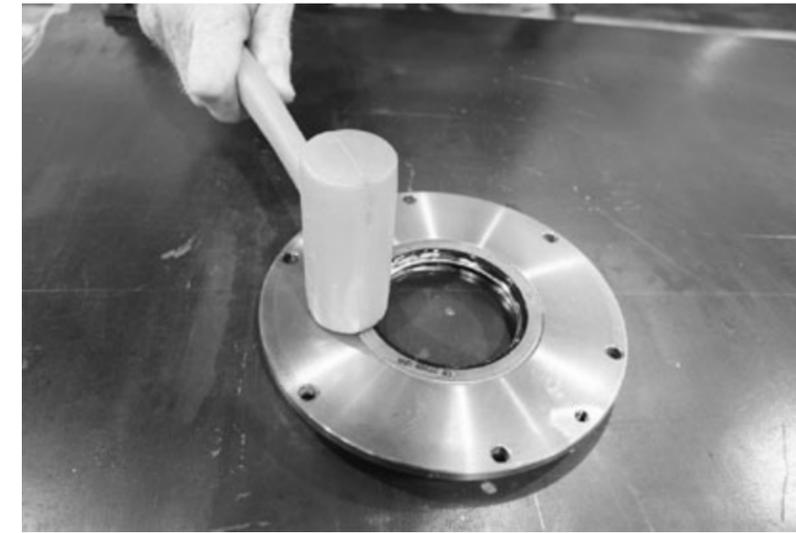
1. Install crankshaft oil seal (VRC28024) into the accessory-end bearing retainer (VRC21120) using a bench press or gently tap the seal into place using a rubber mallet.
