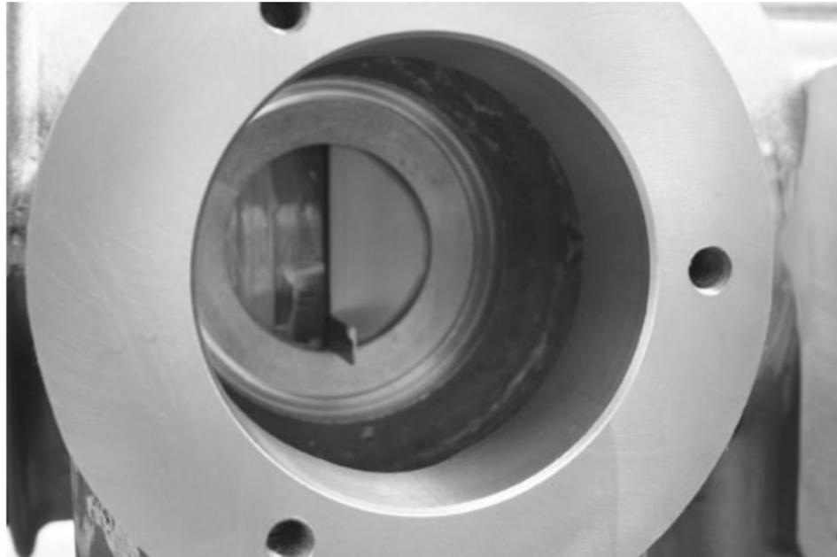
Inset a 0.046" feeler gauge between the piston and the crank-end head to set the clearance correctly.
