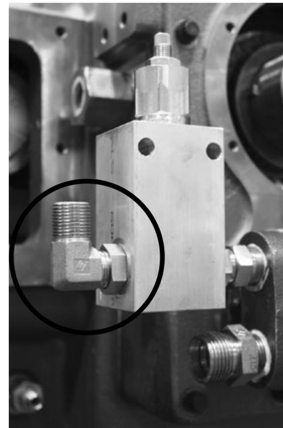
4. Install the relief valve to filter fitting (VRC28815) in the outlet of the relief valve with the 90° outlet pointing up.
