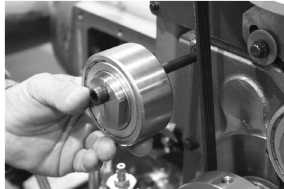
1. Using the housing and idler screw (VRC28067) and tightening with a 5/16" allen wrench, fasten idler bearing assembly to the housing.
