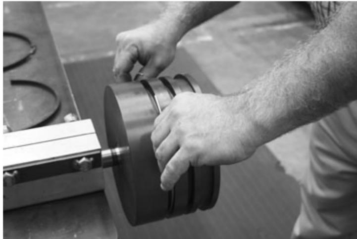
9. Install piston rings and recessed wire expander. Expand the ring with your fingers and slide the ring over the piston to the narrow ring grooves.
