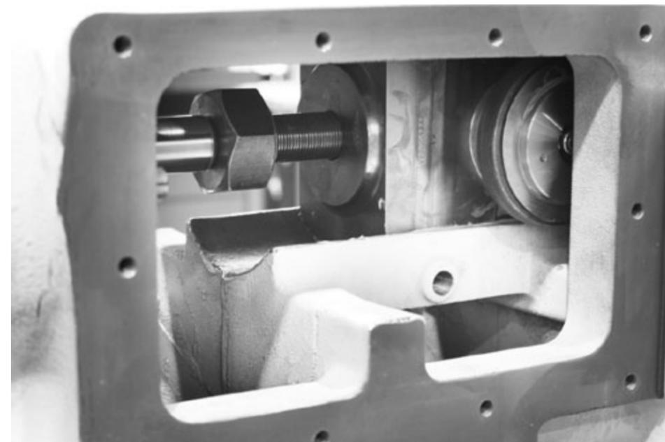
9. Continue to insert piston and piston rod assembly until it begins to thread into crosshead.
