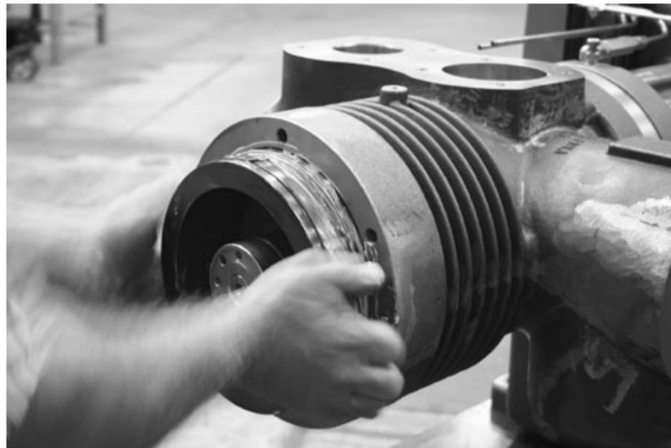
5. While your fingers are compressing the piston rings, carefully insert the piston and piston rod assembly into the cylinder bore (the cylinder is normally mounted to the frame prior to this step).
