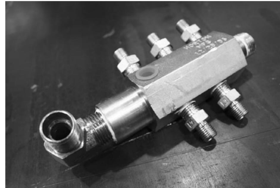
1. Install five (5) 1/4" fittings (VRC28821) into the three (3) ports at the top of the manifold and in the two (2) ports at the bottom of the manifold. Install the 1/2" 90° fitting (VRC28853) at the end of the manifold pointing out from the accessory end.
