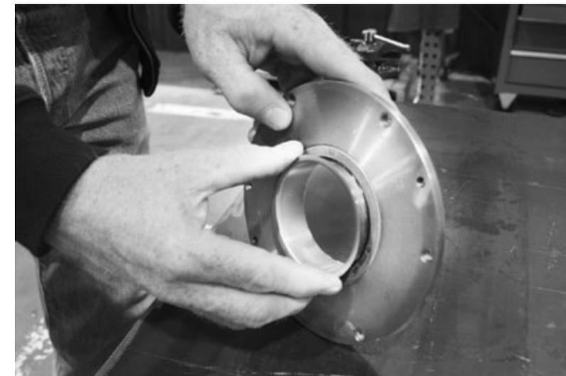
4. Using the special tool, oil seal entering sleeve (VRC29482), insert the tool into the seal.
