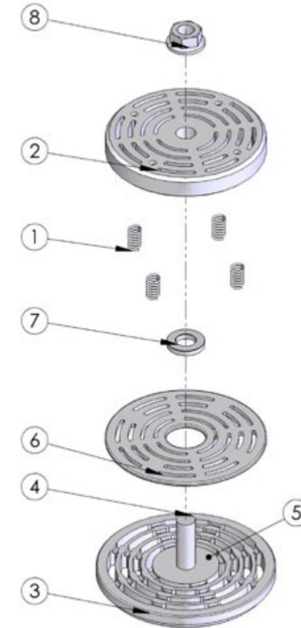
**NOTE:** Arrow Valve Repair Kits do not include valve seat gaskets. It is recommended that new valve seat gaskets be used every time a valve is installed. Refer to the specific cylinder size assembly parts list for "Gasket, Suction & Discharge Valve Seat" part numbers.
