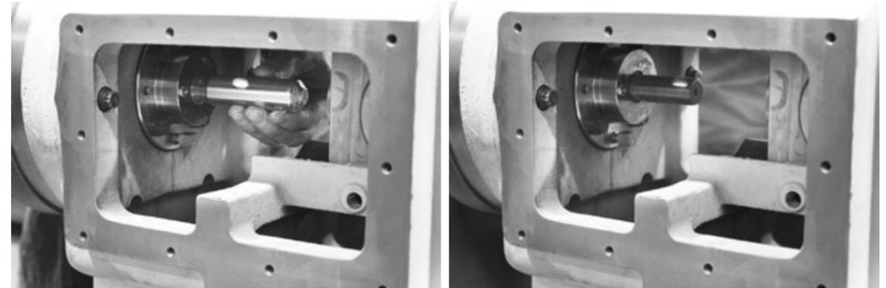
7. Remove entering sleeve tool from rod.
