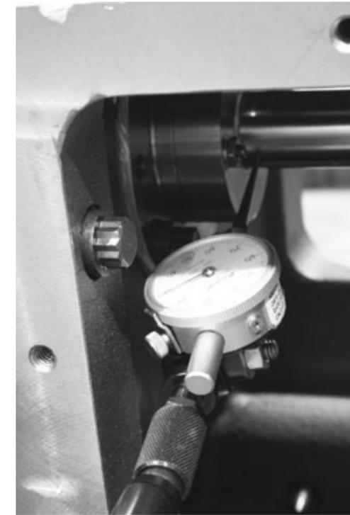
1. Once the dial indicator is in the proper position and is zeroed out, check to make sure the dial indicator is not touching anything that might give an incorrect reading.
