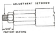
Figure 10.8 - No-Flow Switch Adjustment Set Screw
