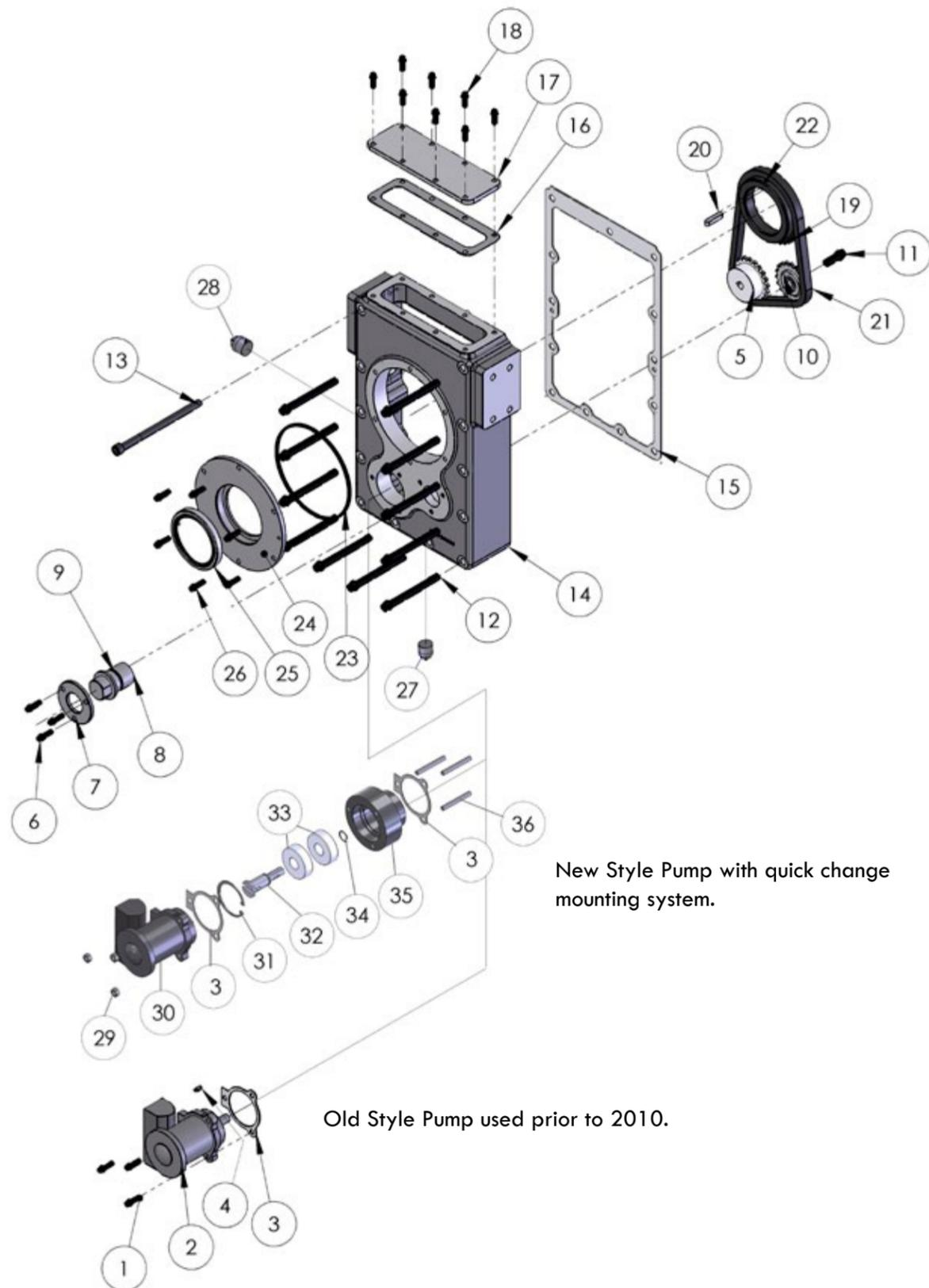
Figure 10.1 - Frame Lubrication System: Chain Drive
