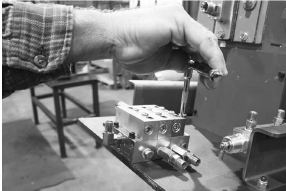
14. Mount cylinder lube oil divider block (see Section 8.4) to the back of the mounting plate using four (4) screws (VRC28607) and tighten.
