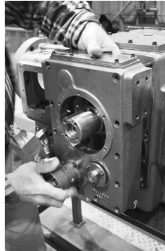
4. Mount the housing assembly to the frame. Make sure that the chain is on top of the crankshaft and push the housing all the way on the frame. Attach the housing to the frame using the housing screws (VRC28007).
