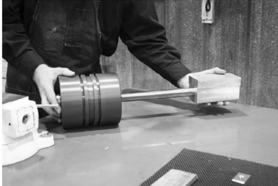
1. Clamp the piston rod in the piston rod clamp device (VRC29494). This device will properly hold the piston rod assembly in place and prevent any damage to the rod.
