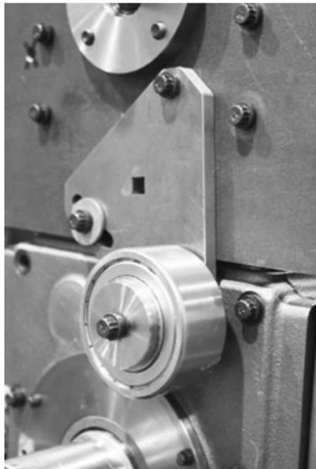
3. Attach the belt tensioner bearing assembly to the adjusting plate.
