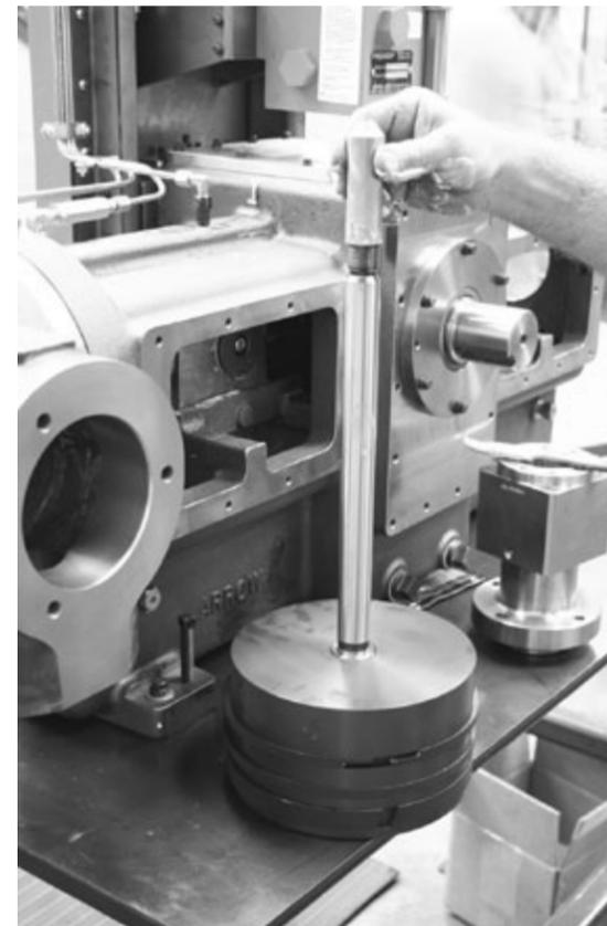
3. Install the piston rod assembly with piston rings into the cylinder. The threaded cross-head end of the rod is 1/8" (3 mm) smaller than the inside diameter of the packing. Its preferred to use an entering sleeve. This Piston Rod Entering sleeve tool (VRC29492) is provided by Arrow.
