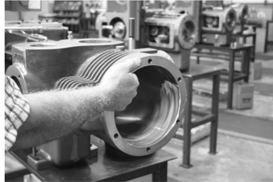
2. Liberally apply lubricant in the cylinder bore.
