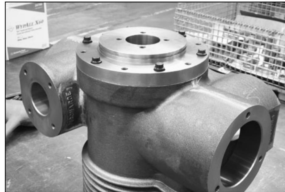
7. Insert 12 screws using a 1/2 inch 12 point socket and torque wrench and torque to 82 ftlbs.
