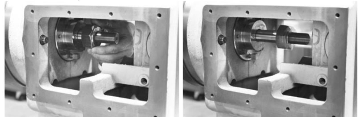
8. Install piston rod jam nut (VRCC4909). Make sure that the raised flat surface of the nut will be against the crosshead.
