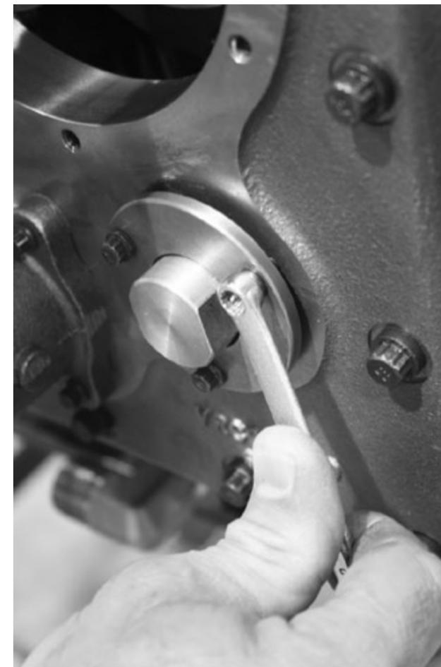
4. After adjustment is complete, tighten screws on the chain idler clamp.
