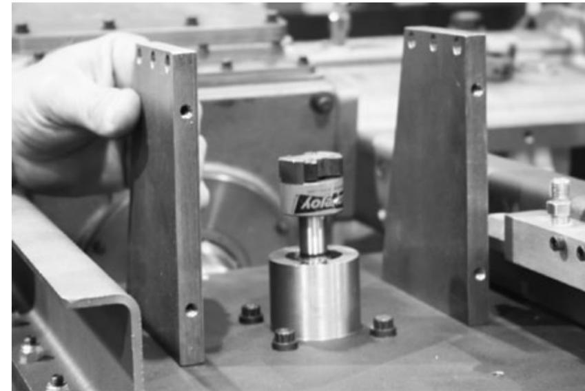
7. Attach the pump support side plates (VRC28572) to the mounting plate using six (6) screws (VC21117) three (3) screws for each side support plate. These screws should be hand tightened and left hand tight until all screws in the supports have been installed.
