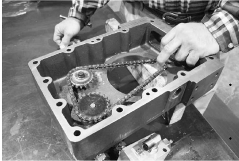
1. After sprocket alignment is complete, install the endless riveted drive chain (VRC28200) over the idler and oil pump sprockets.
