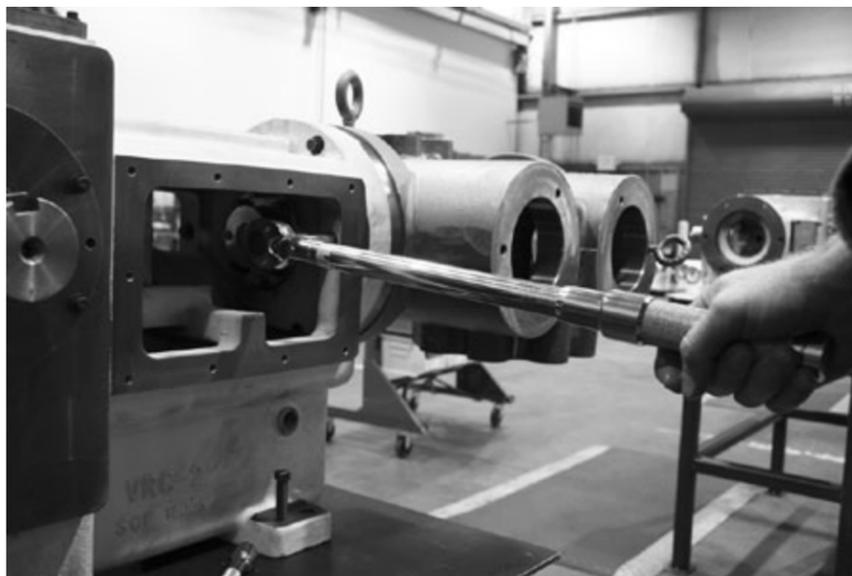
3. Torque the cylinder to frame screws to 82 ftlbs.
