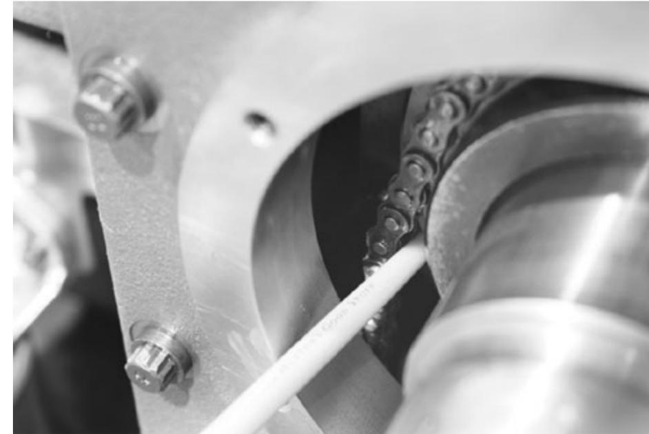
3. Turn the idler clockwise (very slight turns) enough to loosen the chain so that there is a 1/4" of play or sag.
