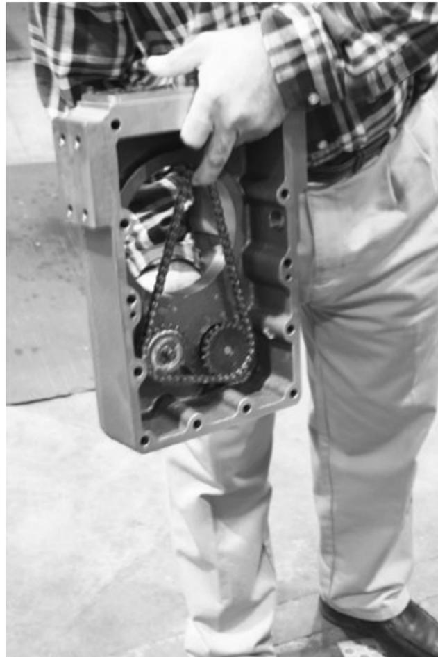
2. Lift drive chain and housing at the same time and prepare to mount the drive chain/housing assembly to the frame.
