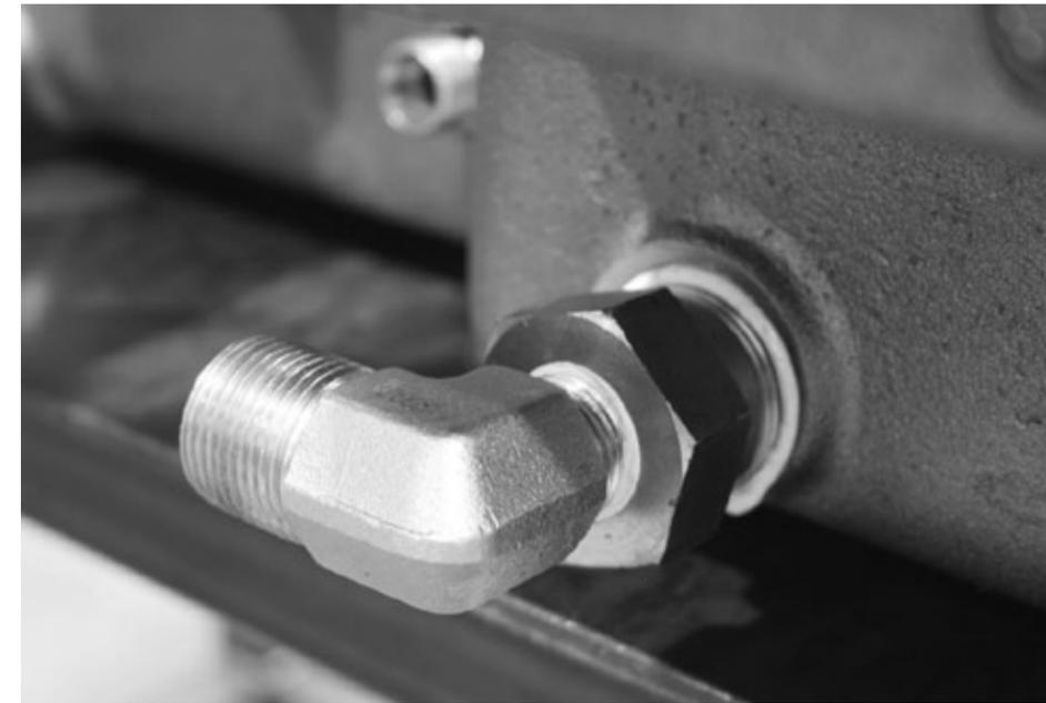
1. Install fitting (VRC28871) into the oil strainer (VRC28340) with the 90° outlet pointing toward throw number 2.
