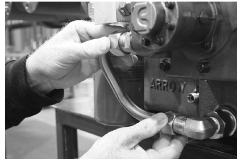
3. Install strainer to pump tubing (VRC28875-13.3) between the oil strainer and the inlet to the frame oil pump.
