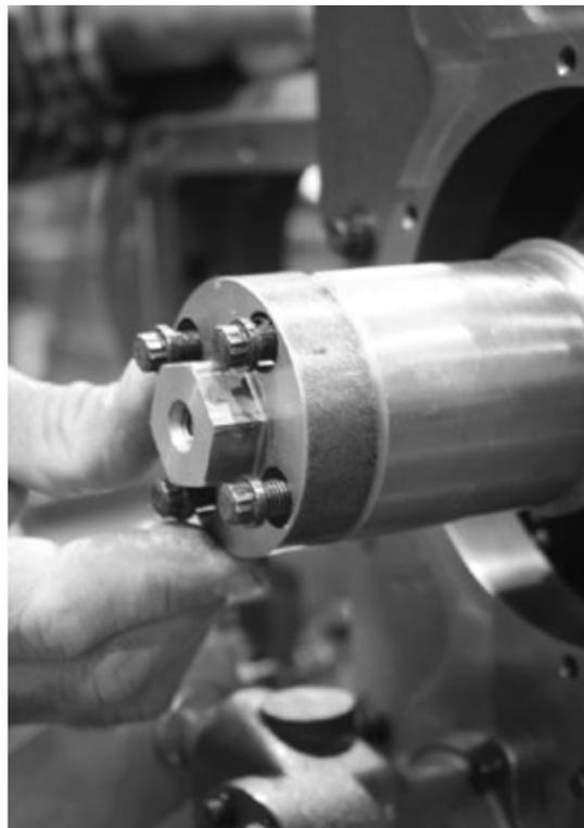
2. Check the slack side of the chain with your fingers then install the crankshaft bar over adapter tool (VRC21140).
