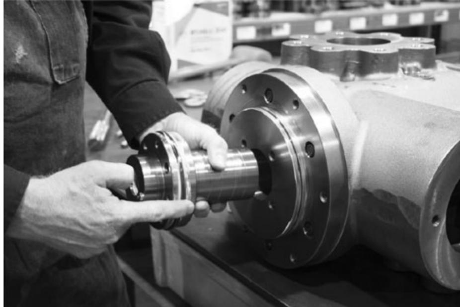
11. Insert packing case making sure the "lube" hole is at the top and the "vent" hole is at the bottom.
