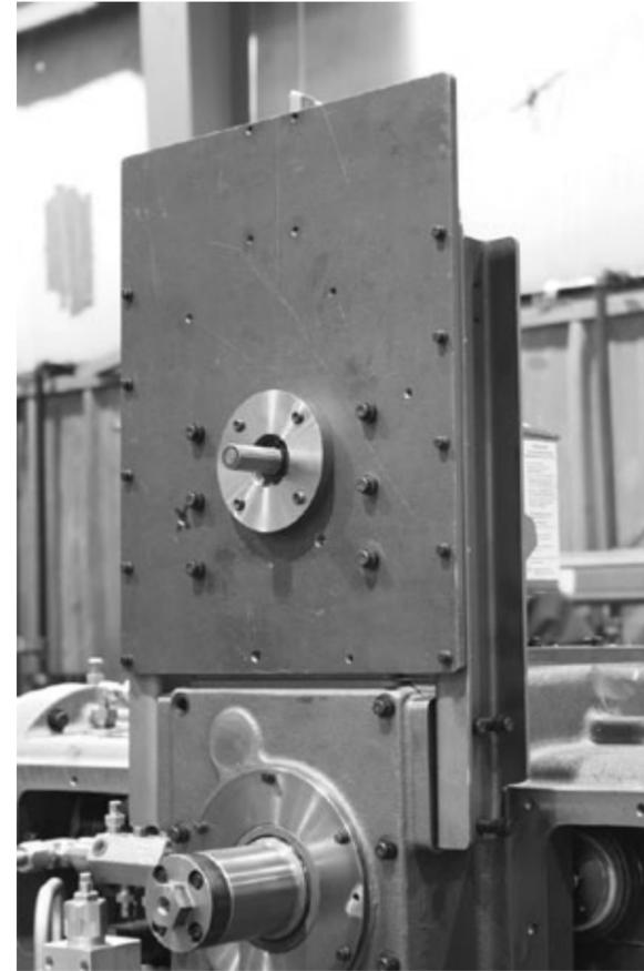
15. Return the housing and mounting plate side supports to the original upright position. Snug (DO NOT TIGHTEN) the mounting plate screws (VRC28557) to allow position of the assembly for proper belt alignment.
