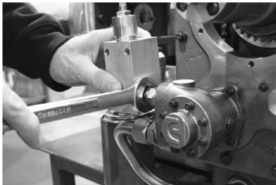
2. Screw the relief valve on to the pump to RV fitting and tighten the lock-nut so that the relief valve is in the upright position.
