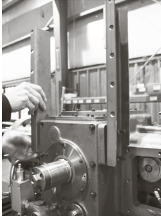
1. Install the Left Mounting Plate Support (VRC28552) and Right Mounting Plate Support (VRC28551) to the appropriate sides of the housing using the plate support screws (VRC28547).
