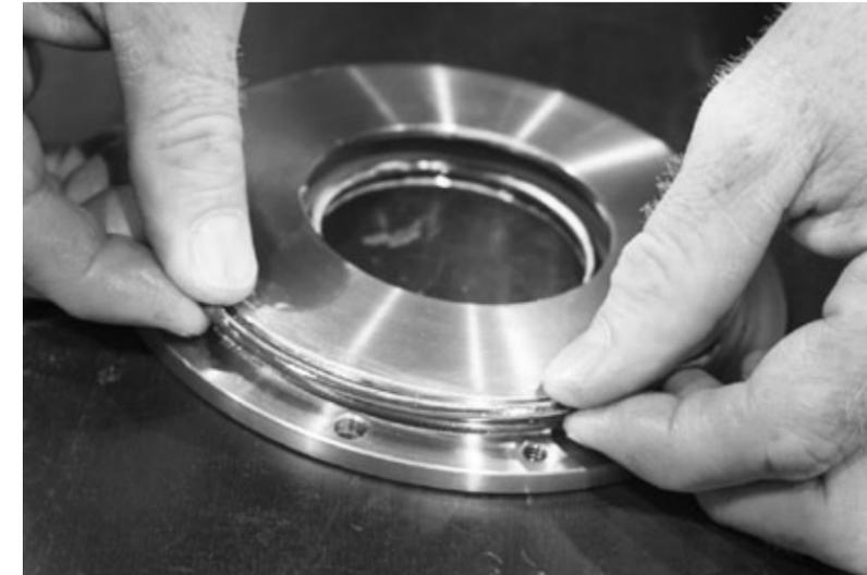
2. Apply lubricant to the oil seal retainer O-ring (VRC28022).
