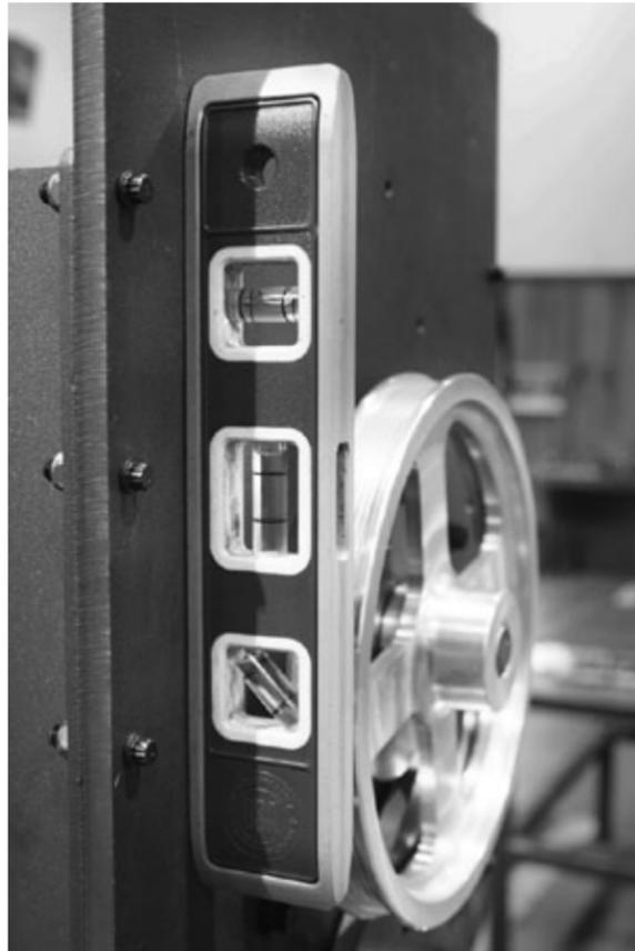
6. Align mounting plate with the face of the drive sheave by placing a level on either side of the mounting plate and observing the position of the bubble.
