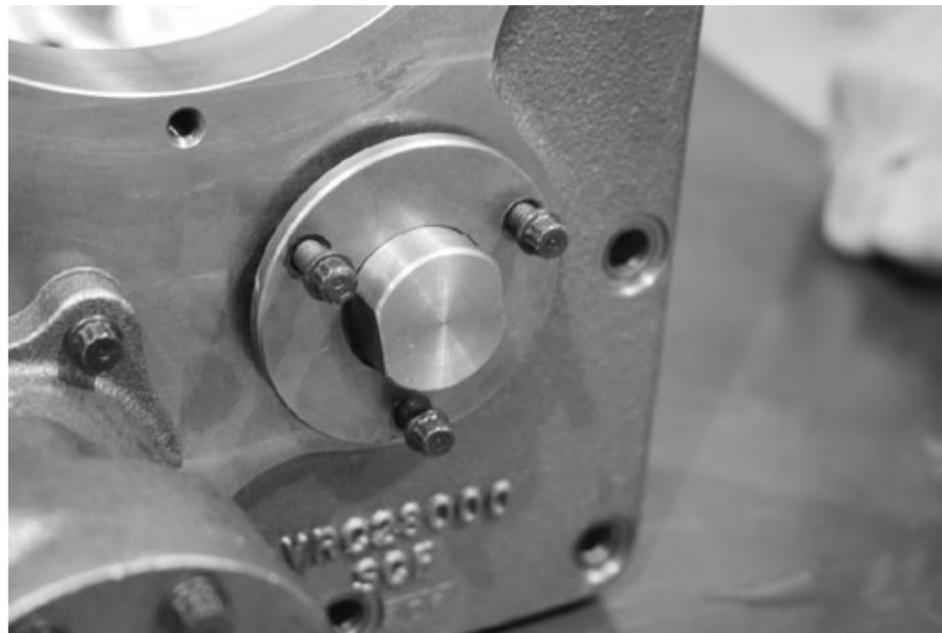
4. Install the chain idler clamp (VRC28253) over the chain idler and secure with three (3) idler chain clamp screws (VRC28257).
