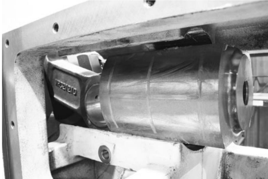
Picture 1 Crosshead flat on side in guide
