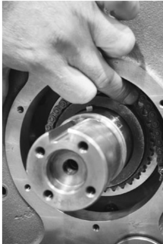
1. Place the chain on the crankshaft drive sprocket.
