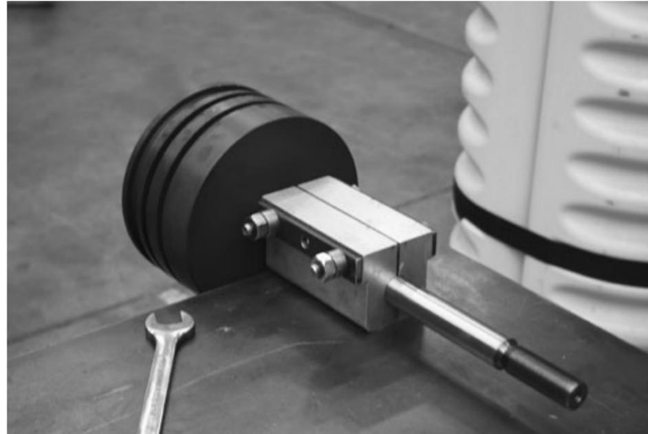
1. Place the 8.5" piston (VRCC4850) on its side and insert the 8.5" x 1.125" piston rod (VRCC4112) in the piston.
