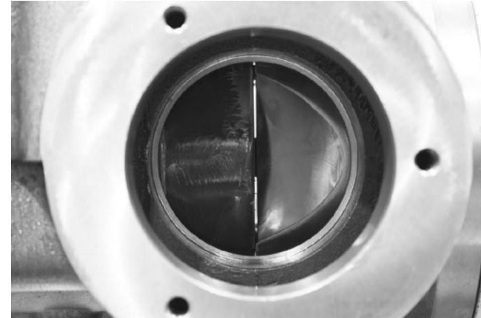
1. Using long feeler gauges, insert .050 feeler gauge between piston and crank-end head. Continue to screw the rod into the crosshead until .050 clearance is achieved. The crosshead must be all the way to the back of its throw at this time.
