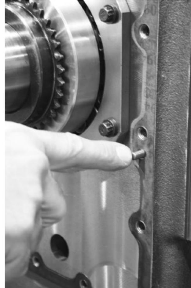
6. Tighten set screw with a 5/32" allen wrench.
