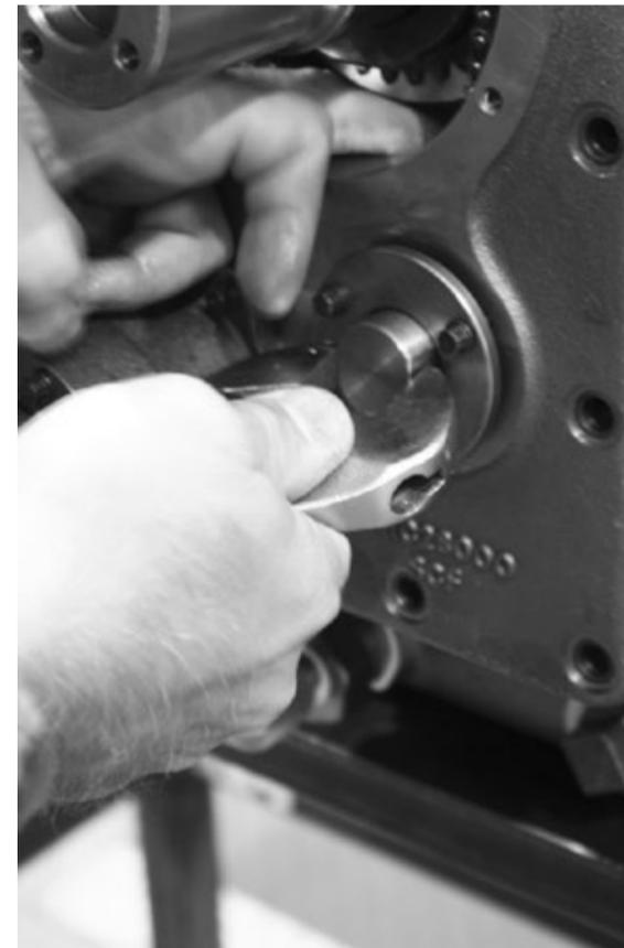
5. With the housing assembly securely in place, loosen the idler clamp screws and turn the idler so that the chain is in its most slack position.
