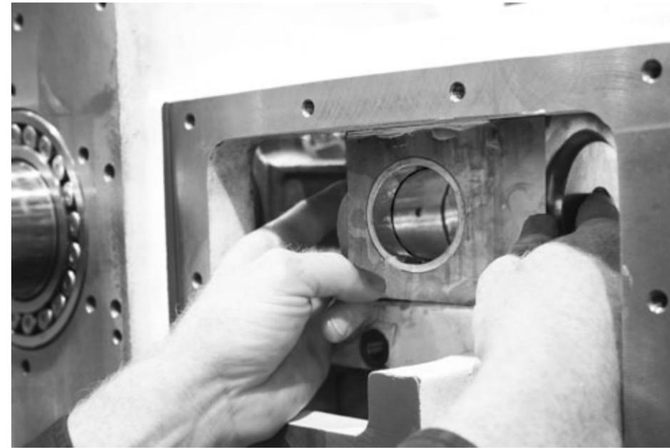
5. Slide the crosshead into position so that the hole in the crosshead is aligned with the hole of the connecting rod. Using your hands, lift the connecting rod so that the hole of the connecting rod lines up with the hole in the crosshead.
