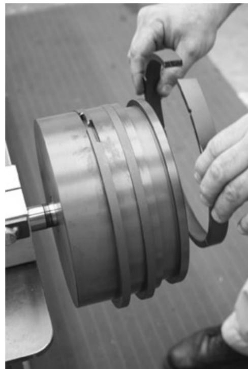
10. Next install the rider band by expanding the band with your fingers and sliding it over the piston inserting it in the wide band groove.
