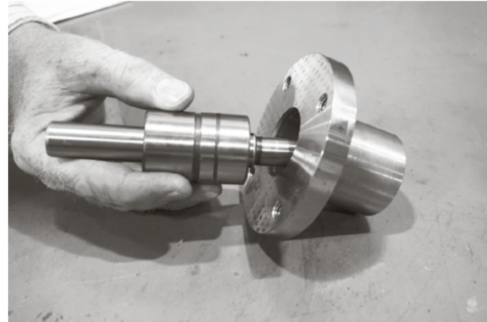
4. Assemble the lube oil pump integral bearing shaft (VRC28581) into the cylinder lube pump mounting flange (VRC28560).
