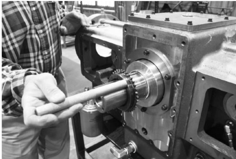
5. Install crankshaft drive sprocket (VRC28248). The teeth of the sprocket should be towards the oil slinger and the integral retainer toward the end of the shaft.
