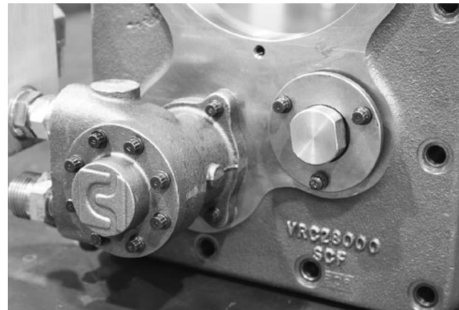
8. Mount frame oil pump (VRC28300A) to housing using the oil pump gasket (VRC28305) and oil pump screws (VRC28307).
