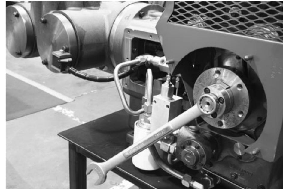
2. Using the crankshaft adapter tool and a 1 1/16" wrench, turn the crankshaft counter-clock wise one full turn (360°).
