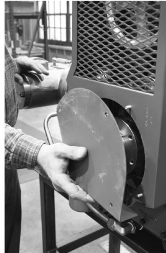
3. Mount the belt guard cover plate (VRC28481) at the bottom of the belt guard using lock nuts (VRC28489).
