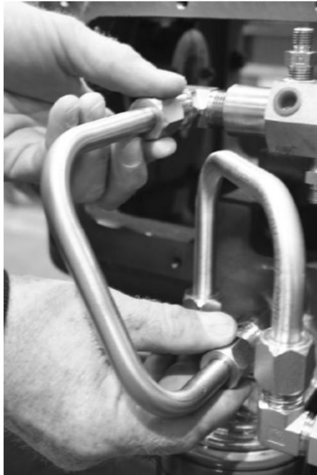
1. Install 1/2" tubing (VRC28850-13.6) between the fitting of the filter bracket and the fitting of the 6 port manifold.
