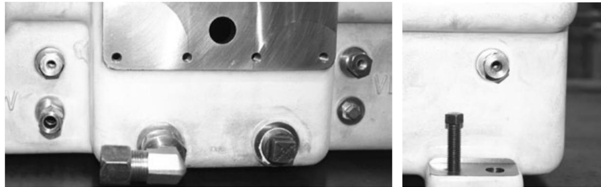
VRC-2 Frame Plugs (VRC21519 and VRC21509)
