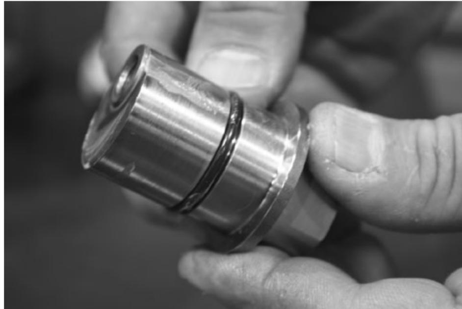
2. Seat the O-ring into the O-ring groove in the frame oil pump idler (VRC28250).
