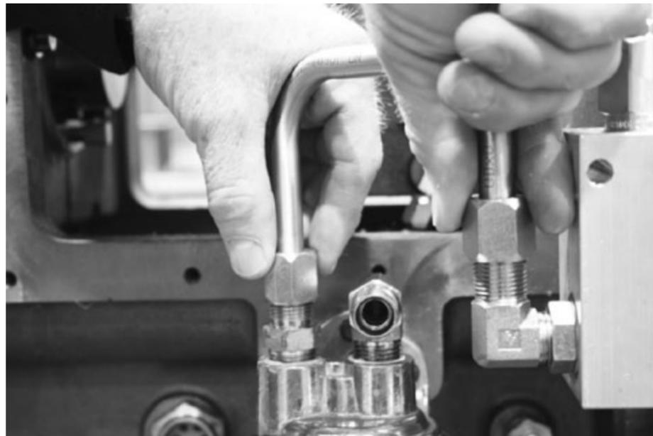
1. Install 1/2" tubing (VRC28850-12.5) to the fitting in the outlet of the relief valve (RV) and to the inlet fitting (VRC28851) of the filter bracket.
