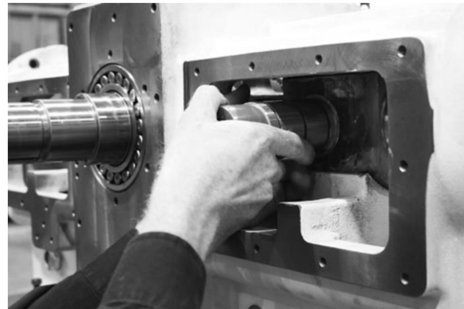
7. Generously lubricate the crosshead pin (VRC22110 or VRC22130) and insert it carefully working the pin into the hole of the crosshead. Make sure the crosshead pin moves freely within the crosshead.
