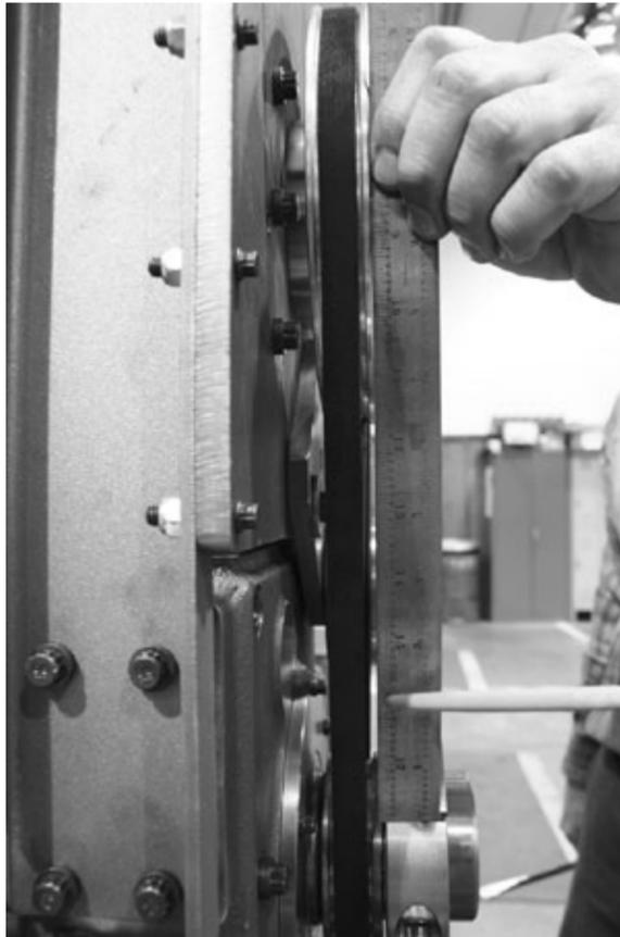
11. Using the drive sheave to make adjustments, move the drive sheave in or out on the crankshaft until proper alignment has been achieved.
