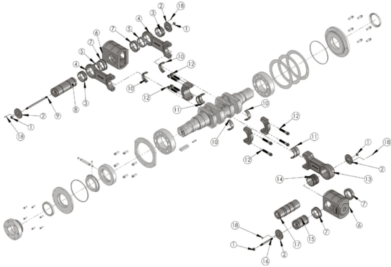
Figure 9.6 - Crosshead and Connecting Rod Exploded View
