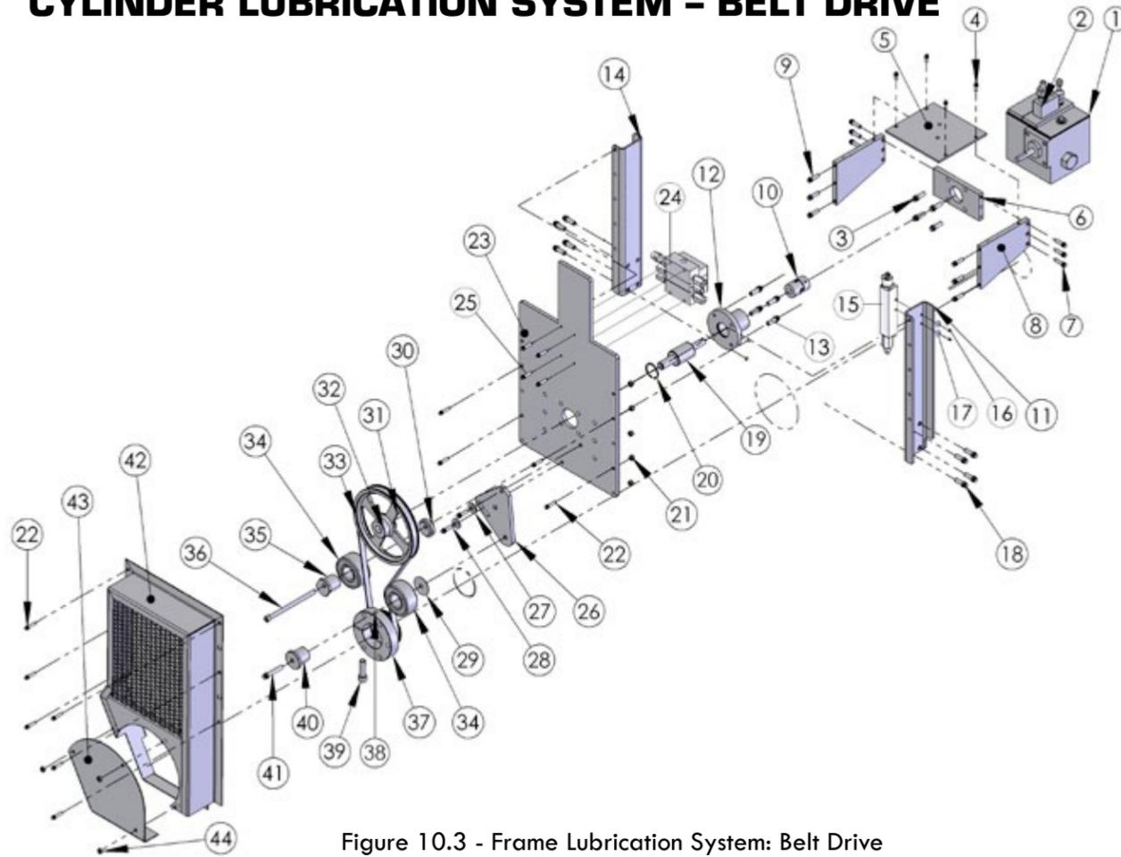
Figure 10.3 - Frame Lubrication System: Belt Drive
