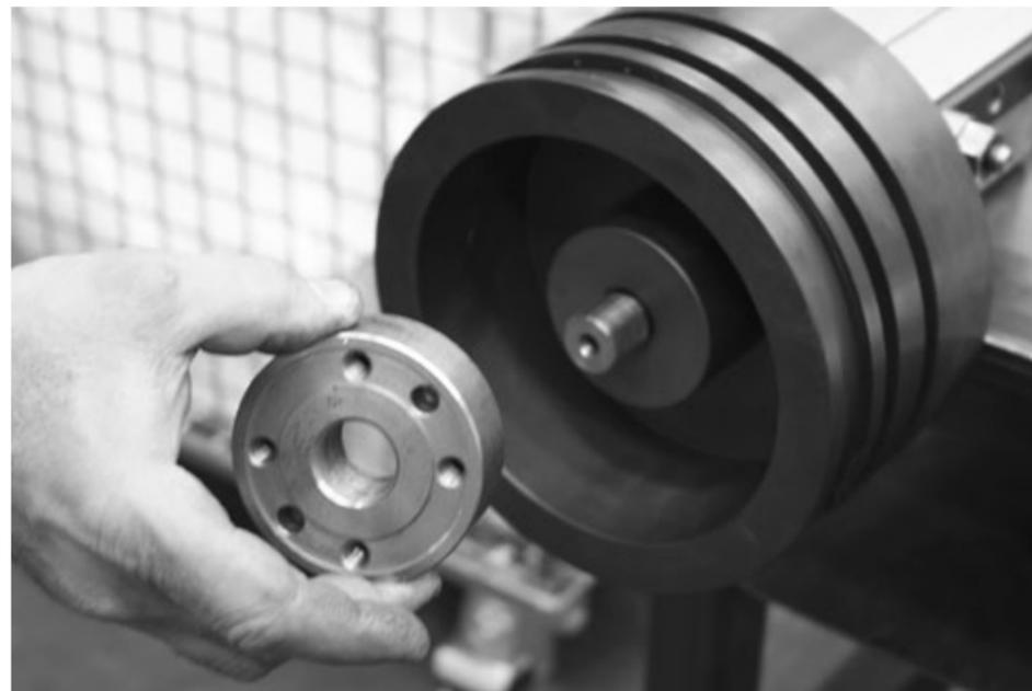
3. Thread the piston nut (VRCC4989) on to the piston rod so that the threaded holes are exposed.
