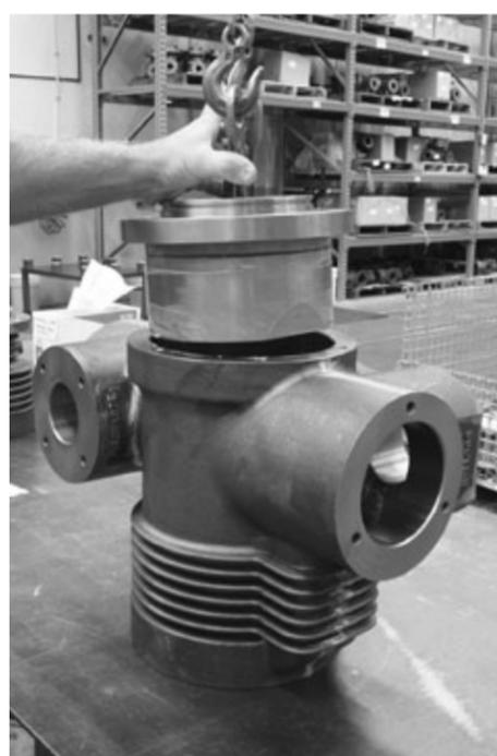
5. Insert the crank-end head into the cylinder.
