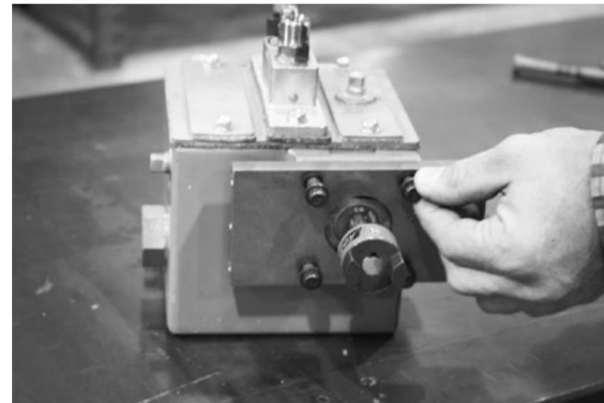
8. Install pump support end plate (VRC28572) to the cylinder lube oil pump (VRC28500) using four (4) screws and tighten.
