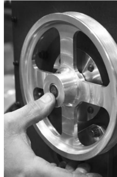
2. Slide the sheave onto the shaft until the end of the shaft is flush with the hub of the sheave.
