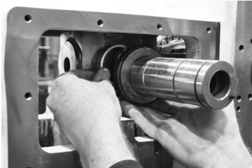
7. Slide the crosshead into position so that the hole in the crosshead is aligned with the holes of each of the two connecting rods. Using your hands, lift each of the connecting rods so that the hole of the connecting rods line up with the hole in the crosshead. Do this for each connecting rod.
