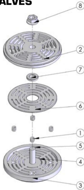
**NOTE:** Arrow Valve Repair Kits do not include valve seat gaskets. It is recommended that new valve seat gaskets be used every time a valve is installed. Refer to the specific cylinder size assembly parts list for "Gasket, Suction & Discharge Valve Seat" part numbers.
