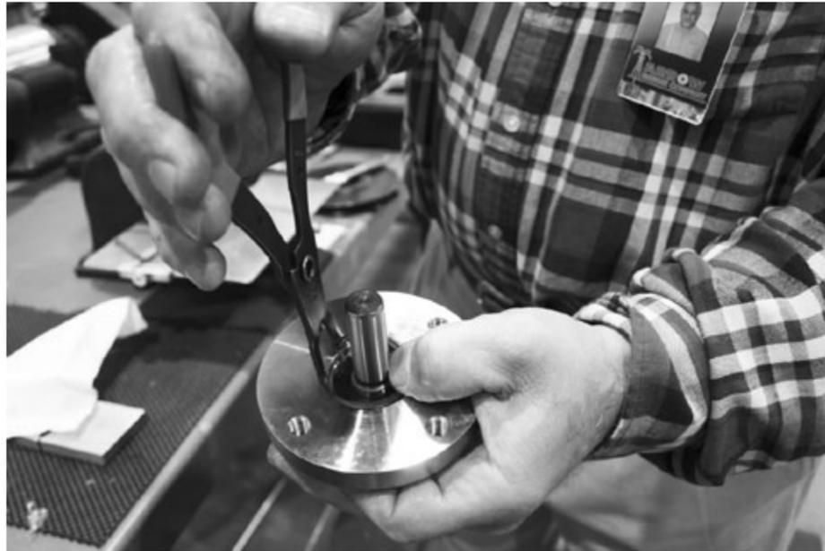
4. Insert pump shaft retaining ring (VRC28583) using snap ring pliers. Make sure the ring properly seats in the groove inside the flange.
