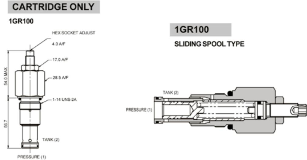
Figure 10.4 - Relief Valve Cartridge Only and Section View
