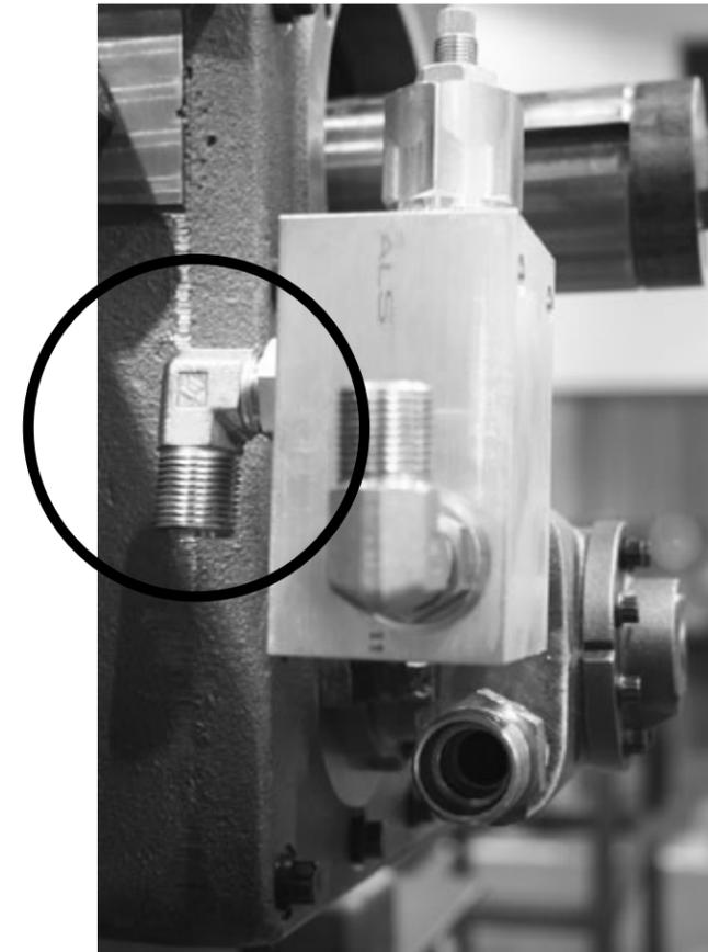
3. Install relief valve (RV) to sump tubing assembly (VRC28812A). Install fitting (VRC28815) in the outlet (Port #2) with 90° outlet pointing down.
