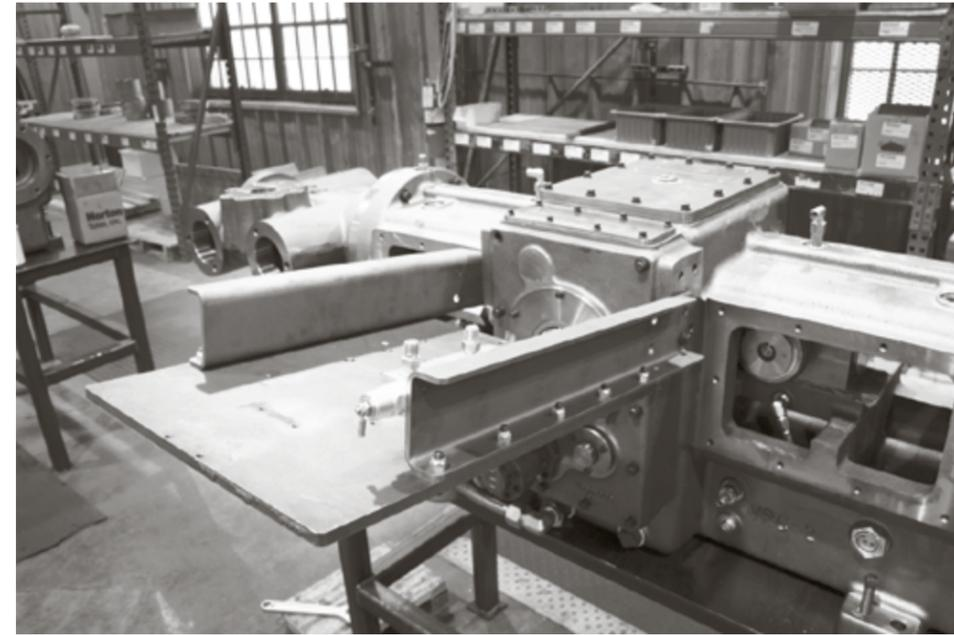
3. Remove all but one (1) screw from each side of the mounting plate support and then angle the mounting plate and support assembly downward. Doing this will make the rest of the belt drive assembly easier to install.
