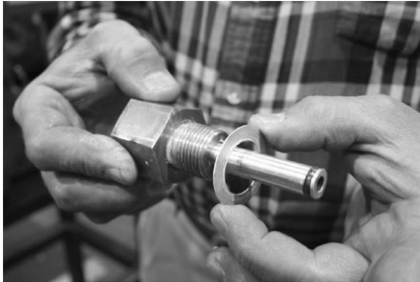
2. Insert the oil slinger tube into the oil slinger tube fitting (VRC28130).
