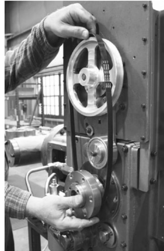
8. Install cylinder lube pump drive belt (VRC28400) over sheaves.
