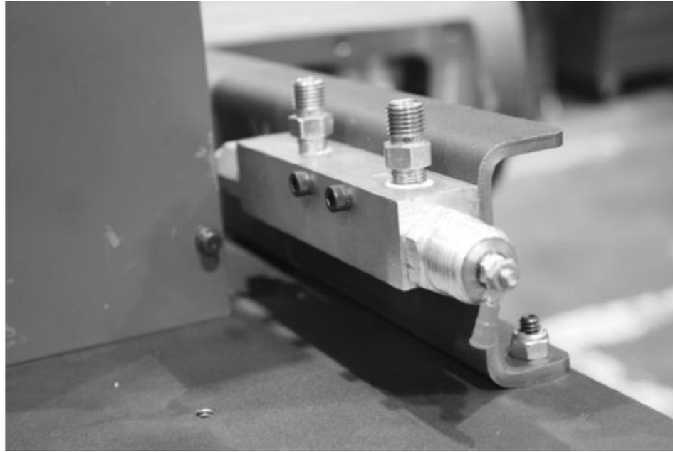
13. Attach no-flow switch (VRC28720) (for more information about the no-flow switch, see Section 10.14) to the right side mounting plate support using two (2) screws (VRC28727) and tighten securely.
