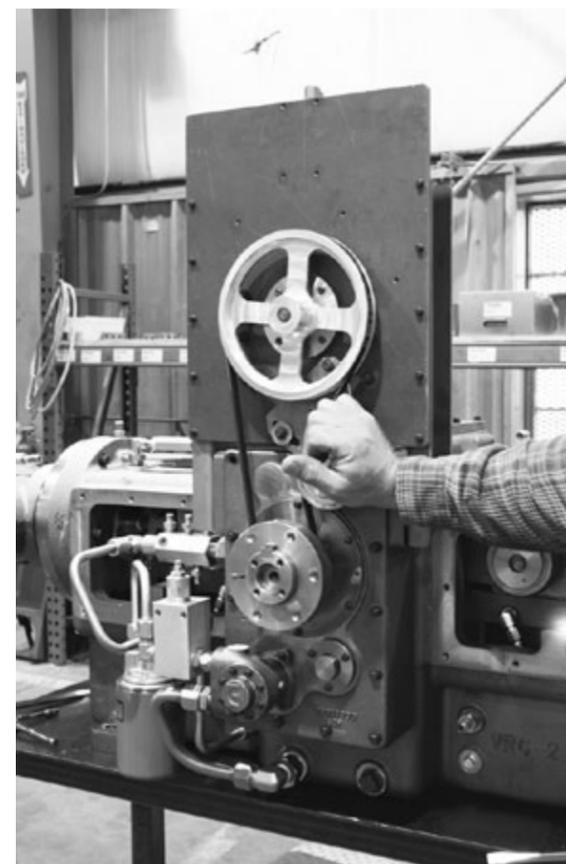
9. Tighten the belt tensioner by putting pressure on the belt tensioner bearing and tightening the adjusting screw. Tighten screw in the belt tensioner adjusting plate.
