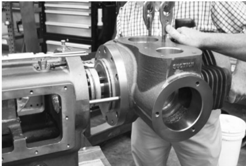
2. Using four (4) screws (VRC25027), cylinder to frame short screws and two (2) screws (VRC25047) cylinder to frame long screws, attach the cylinder to the frame.
