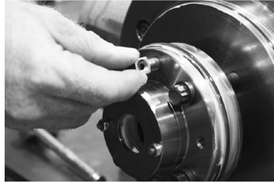
15. Apply anti-seize to threads of fitting and insert fitting into packing case in the "lube" hole.
