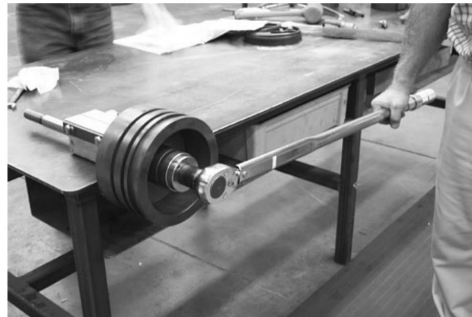
5. Insert the piston rod into the rod clamp (VRC29494) and place both into a vise and tighten firmly.
