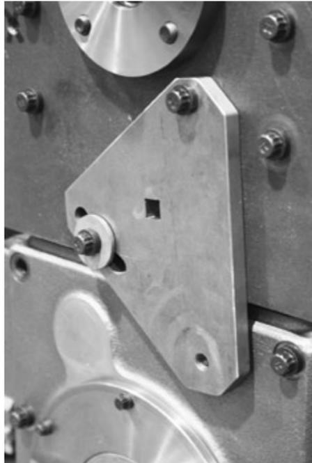
2. Mount the belt tensioner adjusting plate (VRC28472) using two (2) screws (VRC21117). There will be one (1) screw at the top of the adjusting plate and one (1) at the slotted adjusting hole using an adjusting plate washer (VRC28476).
