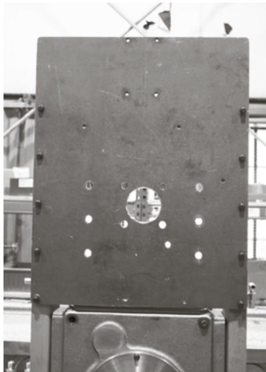
2. Attach the mounting plate so that the tapped holes for the belt tensioner are on the right hand side (right hand side as you are looking at the accessory side of the compressor). Attach the mounting plate to the supports using the mounting plate screws (VRC28557) and mounting plate lock nuts (VRC28550).
