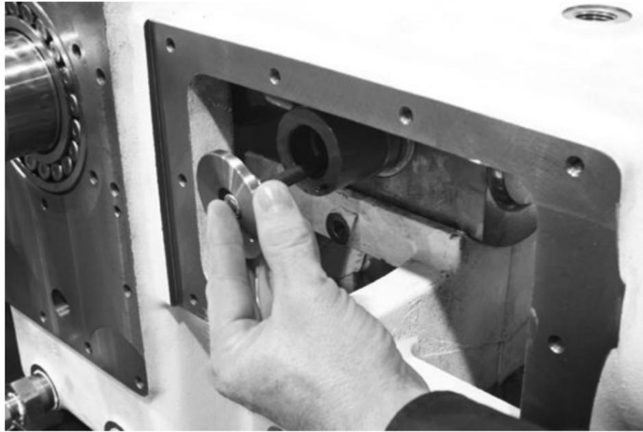
7. Install the retainer caps, through bolt stud and locknuts. Torque the locknuts to 25 ftlbs.
