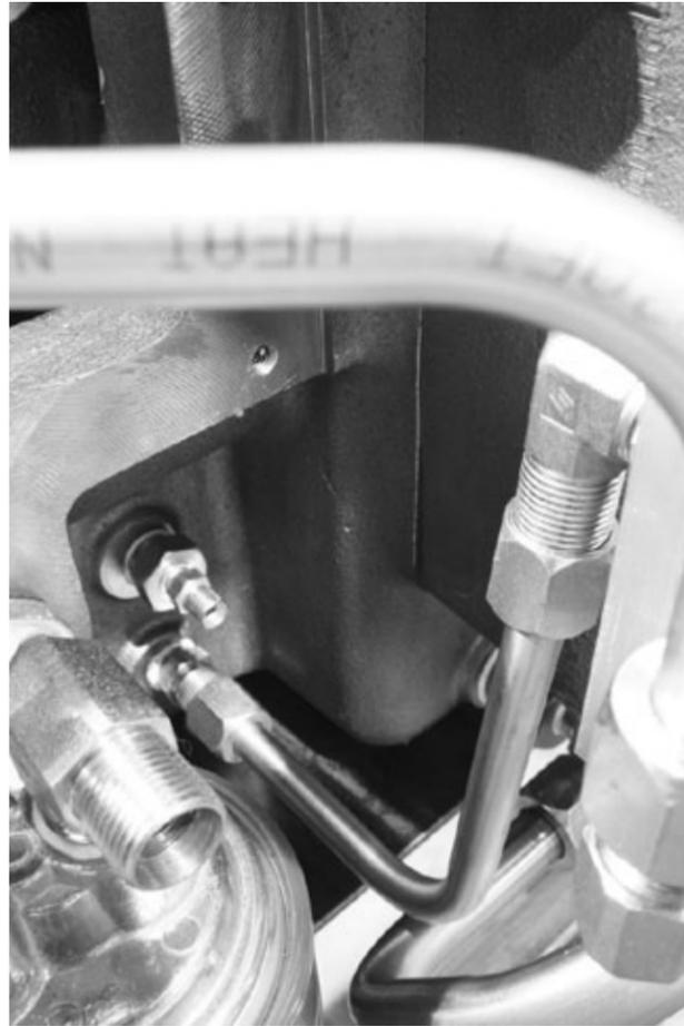
Install 1/2" tubing (VRC28850-10.7) by attaching it to the relief valve (RV) to sump fitting (VRC28815) on the relief valve and to the fitting at the bottom of the frame sump (VRC28852).
