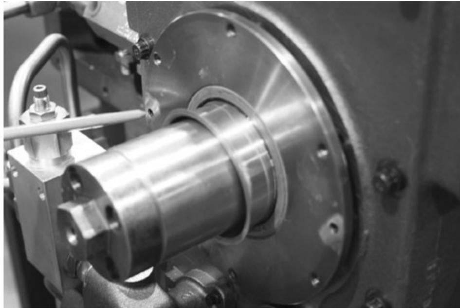
2. After installing the retainer, remove the oil seal entering sleeve tool.
