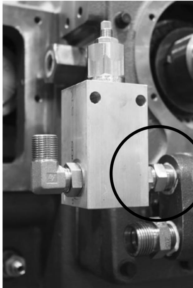
1. Install the pump to relief valve (RV) fitting (VRC28801) in the inlet of the top outlet hole of the pump. (For more information regarding the relief valve, see Section 10.6)
