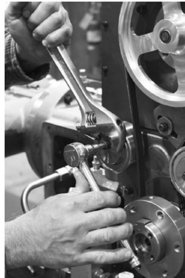
2. Position idler by using eccentric adjuster and apply only slight pressure to the belt. Bearing should be able to turn by hand.
