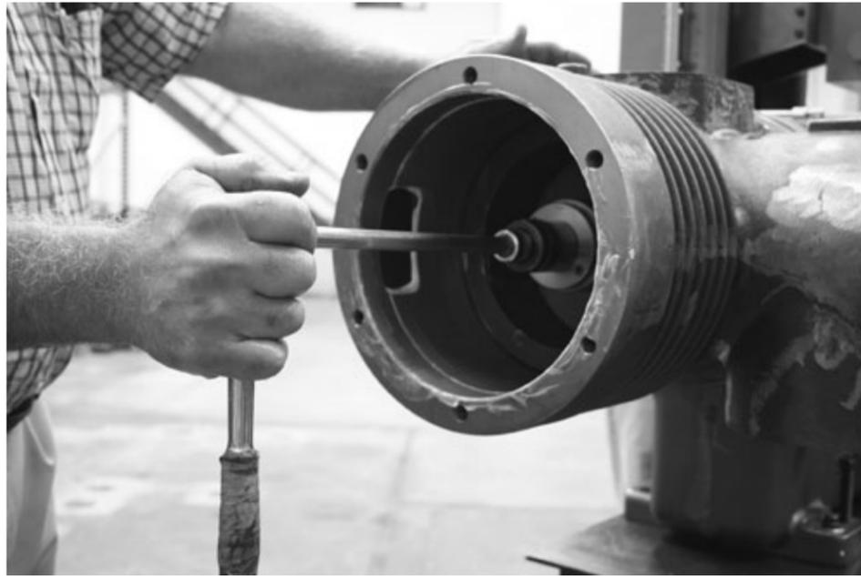
10. Using the piston nut adapter tool (VRCC9490) screw the piston and piston rod assembly into the crosshead while the crosshead is all the way to the back of its throw.
