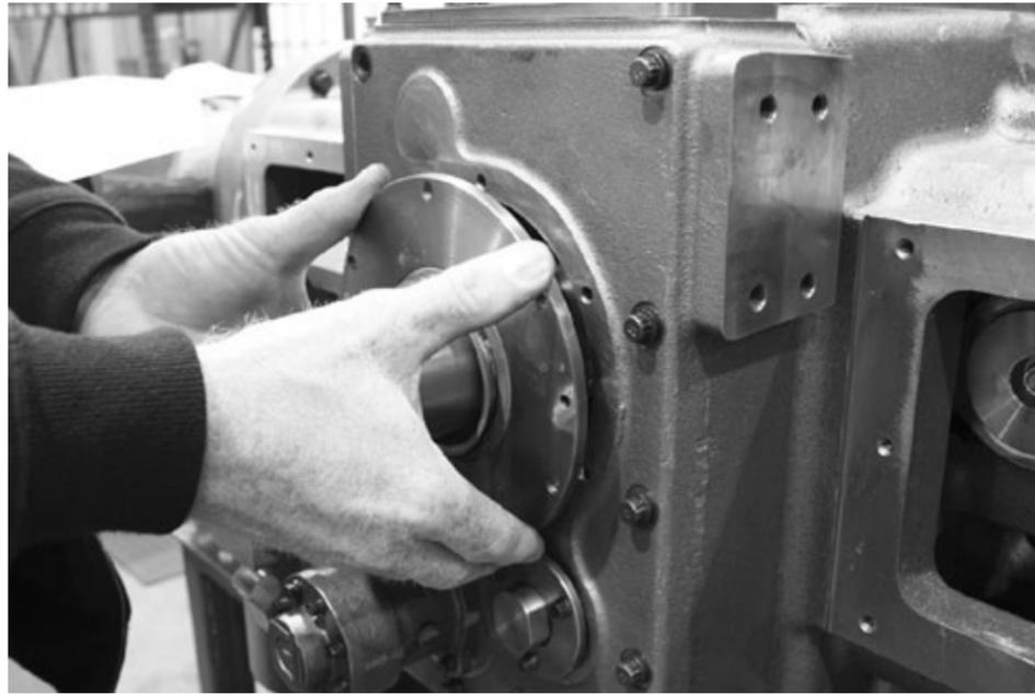
1. Carefully slide the retainer on to the shaft installing the retainer so that the retainer puller holes are positioned horizontally.
