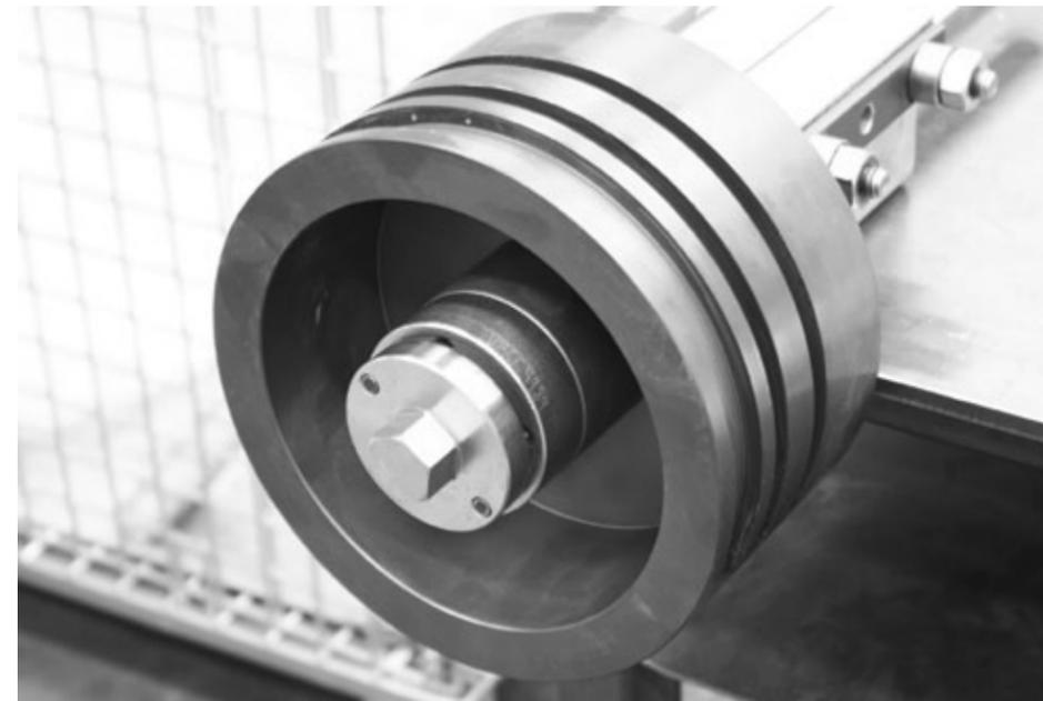
nut by hand. Then using the piston nut adapter tool (VRCC9490), insert the pins of the adapter into the holes of the piston nut.
